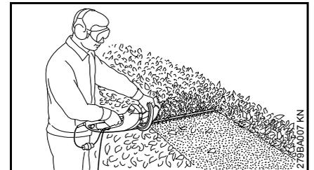
If the hedge is wide, cut it in several passes – one hand on the front switch lever – one hand on the control handle.
