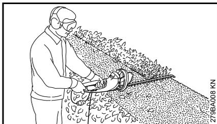
To extend your reach, hold the control handle with one hand and operate the auxiliary switch at the rear of the control handle with the other hand.
