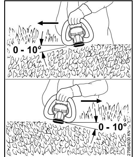
Hold the cutting blade at an angle of 0° to 10° as you swing the hedge trimmer horizontally, using both sides of the blade.
