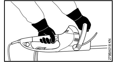
Left hand on the control handle and right hand on the loop handle.
